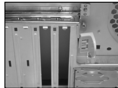
Fastener Figure. Push down here to lock the fastener
